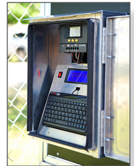
Standard CMS units are equipped with an on-board keyboard for programming and NTCIP Compliance.
