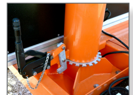
Gear style braking system secures the display angle.
